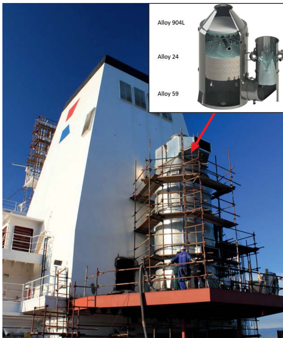
Hempel suppliers Alloy 24, 904L (1.4539) and Alloy 59 (2.4605) for scrubber technology designed in German and built in China. Pictures courtesy of Saacke GmbH
